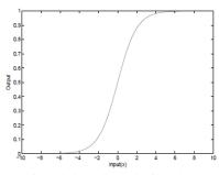
Fig. 2. Shape of a original sigmoid function
