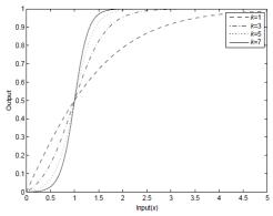
Fig. 3. Sigmoid curves with different ks (B) Noise suppression
