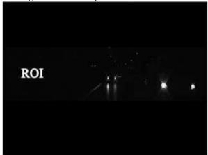
Fig. 6. Intensity image with region of interest (A) Bright object segmentation
